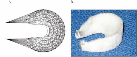
FIGURE A. THIS UNIQUE FIBER NETWORK DESIGN ENABLES THE SCAFFOLD TO SUPPORT MECHANICAL LOADS IN THE KNEE
